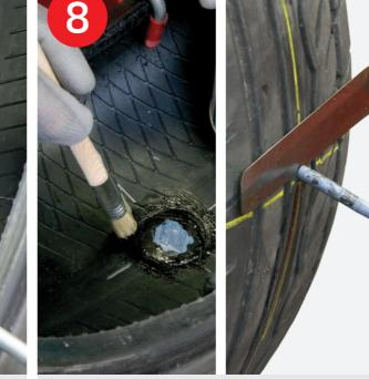
Seal the MINICOMBI base and any still exposed buffed areas with INNERLINER SEALER and cut the stem.
