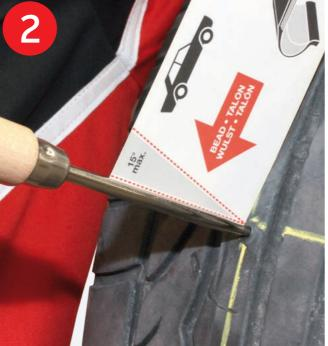
Determine the direction of the puncture channel.
