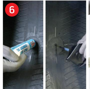
Apply CEMENT FD-BL on the buffed surface, fill the puncture channel with fresh cement and immediately insert the MINICOMBI plug.
