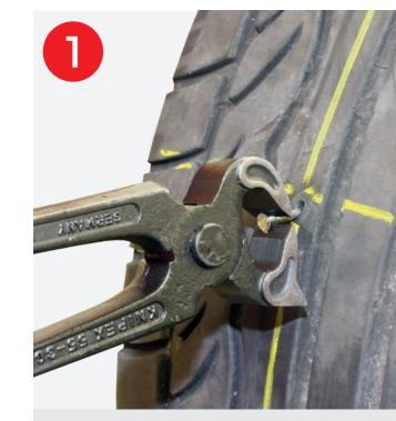
Locate and mark the damage. Take or screw out the foreign object.
