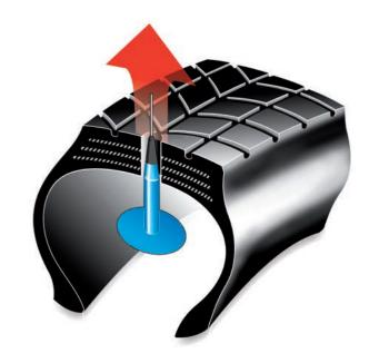
Maximum number of repairs carried out with MINICOMBI repair plugs in one tyre. Always check whether repairs already carried out in the tyre are defective. Axial distance between repairs: minimum 15 cm/6".
