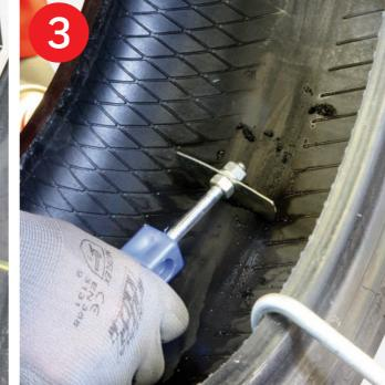
Clean the repair area using LIQUID BUFFER and a scraper.
